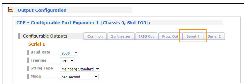
Figure: Menu Tab "Serial 1/2" Setting of the parameters for the serial port
